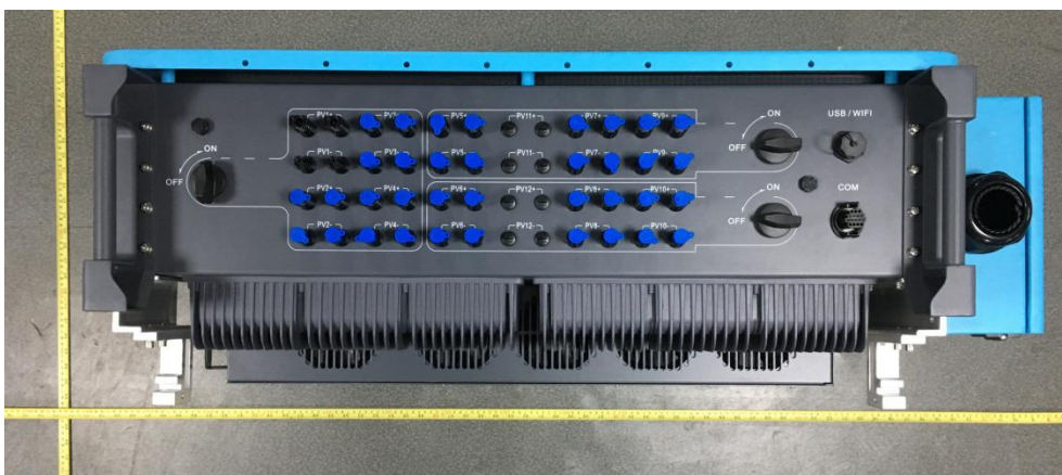
DC connection interface (E-100KTL, E-110KTL, E-100KTL-HV, E-125KTL-HV)
