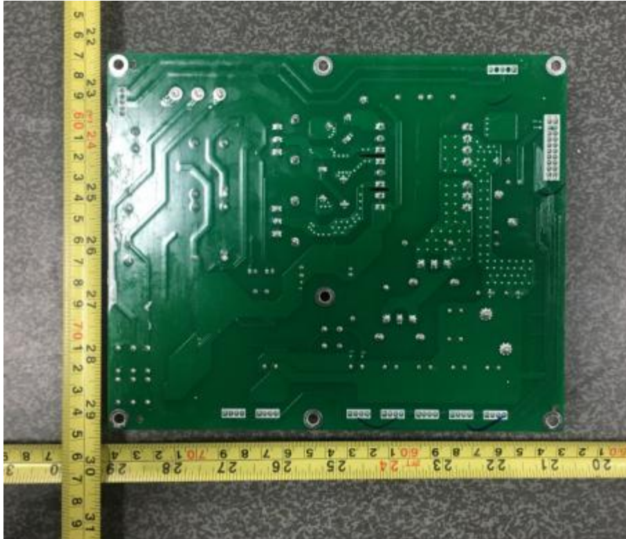
The back of power circuit board
