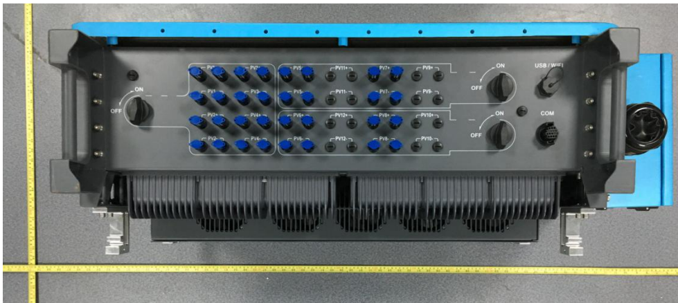
DC connection interface (E-75KTL, E-80KTL)
