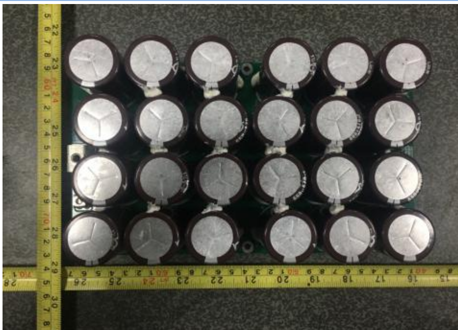
The front of BUS capacitor board
