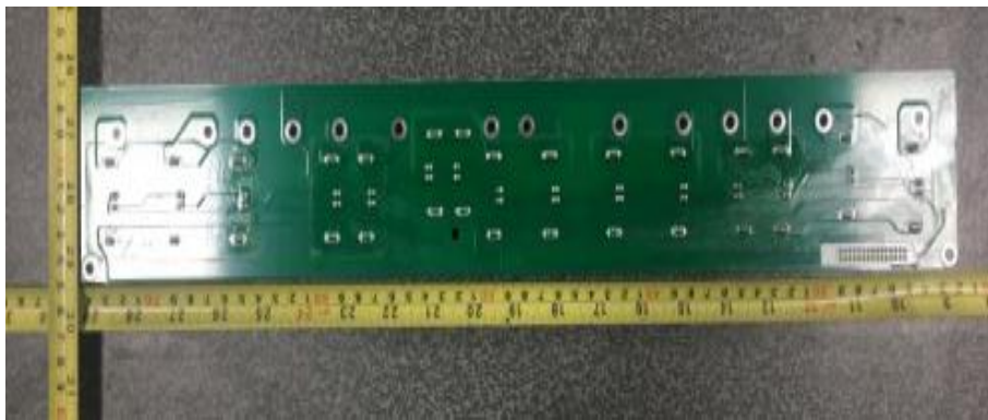
The back of lightning protection board
